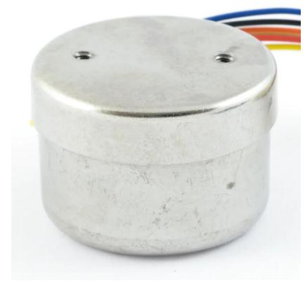
frequency response and minimal phase distortion. Mumetal core for minimal harmonic distortion. Internal electrostatic shield to ensure a fully balanced output at high frequencies. Mumetal can for magnetic shielding.
